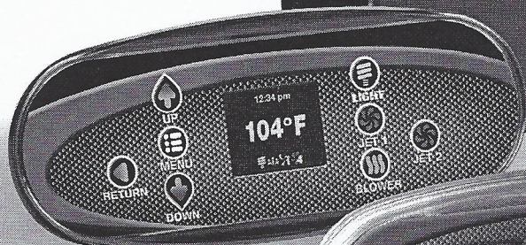
NEO 2100 CONTROL PANEL
